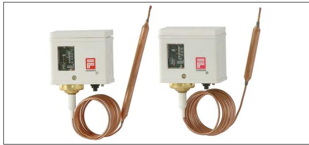
T series temperature control is a temperature-controlled electric switch, can be directly connected to single-phrase A.C. motors of up to about 1KW, or installed in the control current circuit of D.C. motors and large A.C. motors.
