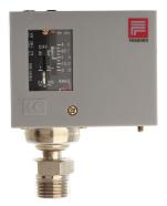
P6W12S pressure controller is a control equipment which is specially designed for fire protection system. Its characteristic is: it not only has a fast working SPDT (single pole double throw) switch, but also can control the low pressure. It can send out the single in a fairly small pressure to make actuators stop working, it protects the pressure well.
